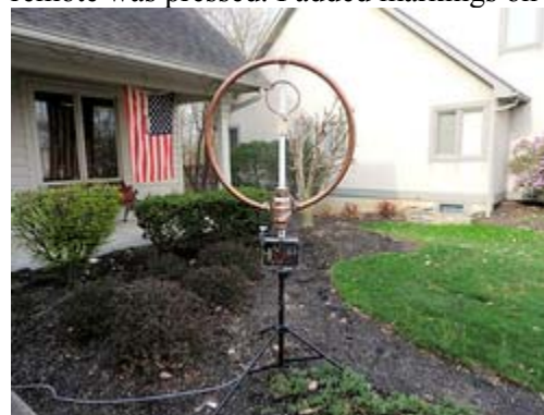
The magnetic loop for 40 and 20 meters designed by Richard Robbins, WA8RR. [Photo courtesy of DELARA News]
