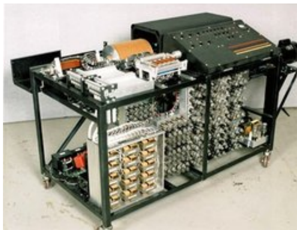
The Atanasoff-Berry computer used racks of vacuum tubes.
